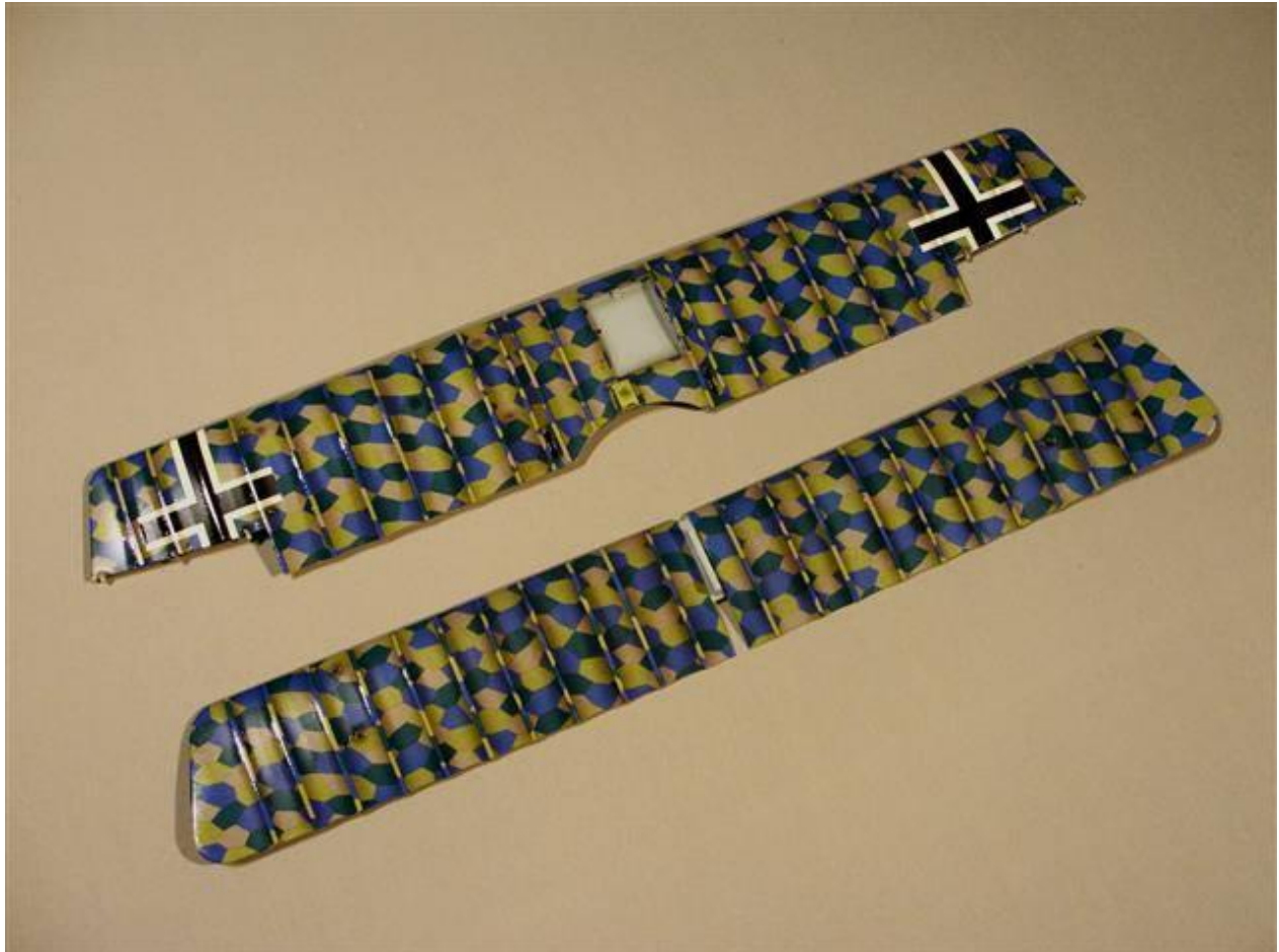
Fig.2) Here's where things start to change already. That's "Clear Black" (Smoke) applied with an airbrush along the rib tape masking. The masking tape has been removed already. We now have emphasized the construction method of the wing. Also we have a remarkable change in appearance already.
