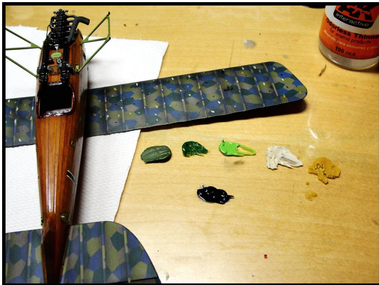
Fig.6) The wings have received a solid coat of flat varnish. I sued flat because we are going to filter the decals now, in order to reduce the unwanted liveliness of the Lozenge decals. We need to “mute” them further and we also should see if we can fade one or the other section a lil bit. This technique is very common amongst armor modelers and sometimes referred as "Fading". We like "break up" the colors now, mute decals and create another layer of “visual texture” using a fast and efficient technique.
